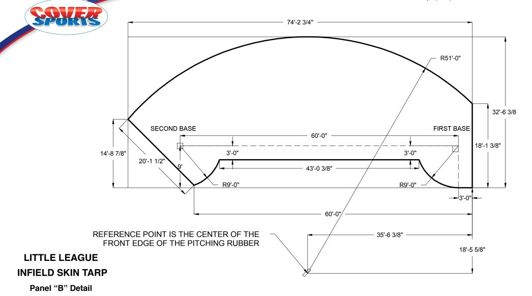
DIMENSIONS SHOWN ARE TO 1/8" PRECISION. ACTUAL PRODUCTION TOLERANCE IS +/- 3 TO 4 INCHES.
