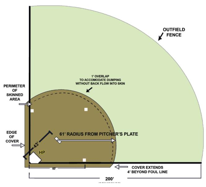
\*NOTE: COVER IS DESIGNED TO BE SLIGHTLY LARGER THAN DIMENSIONS FOR SKINNED INFIELD AREA AND WILL OVERLAP ONTO TURF. DESIGN ALLOWS FOR RAINWATER ON TOP OF COVER TO BE DUMPED ON TURF WHEN REMOVING COVER AND PREVENT BACKFLOW ONTO SKINNED AREA.
